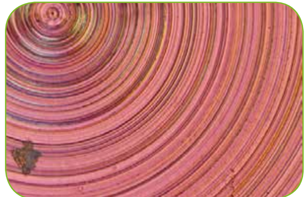
Detail of machined aluminum image with DIC module
