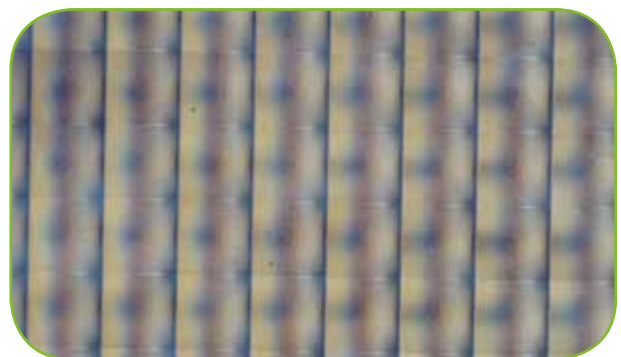
Micro lens array in DIC mode
